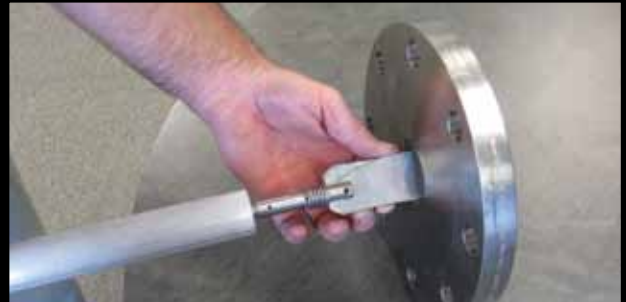
The paddle automatically springs open after it is through the wall.
