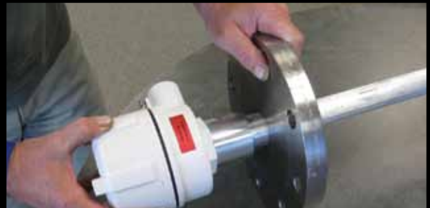
The rotary can then be mounted by screwing it into the coupling or mounting plate.
